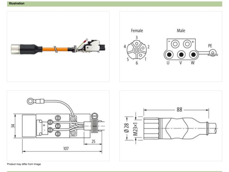
Cable length16 mSide 1Tightening torque2 NmFamily construction formM23ThreadM23 x 1Width across flatsSW27
